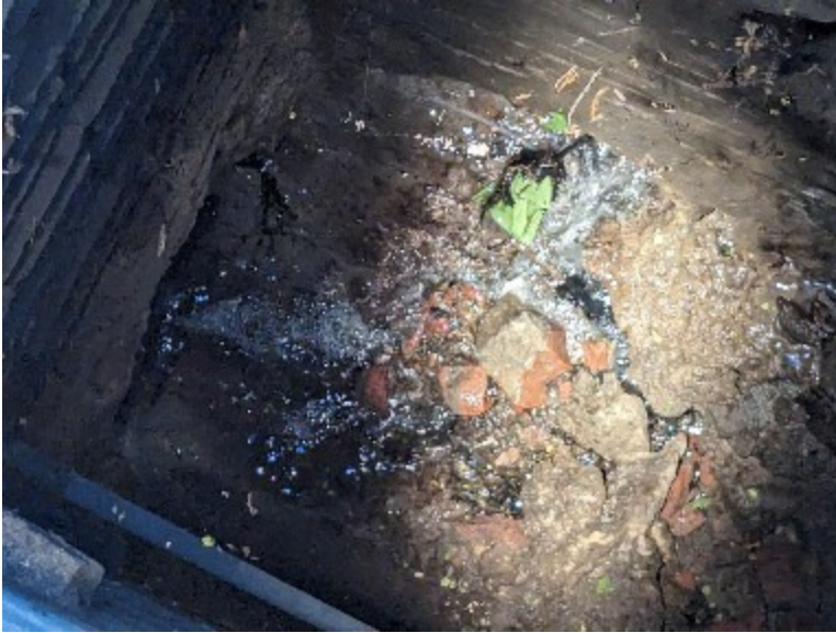
8. CB-3 Ernest connect to COMB-B (green dye)
